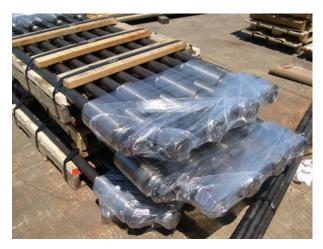
This picture shows the sixteen bars to be threaded thru the plate on the drawing. The fabricated plate circles are 130" +/- 1/4" dia and are flat within 1/8".
